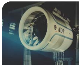
ADP Demonstrator Advanced Ducted Propfan 1993; 50klb Schub
