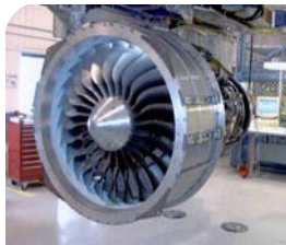
Advanced Technology Fan Integrator, ATFI Geared Fan Demo 2001; 13klb Schub
