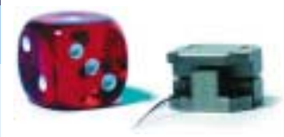
Novel piezo electric motor for nanopositioning (attocube systems AG, Munich)
